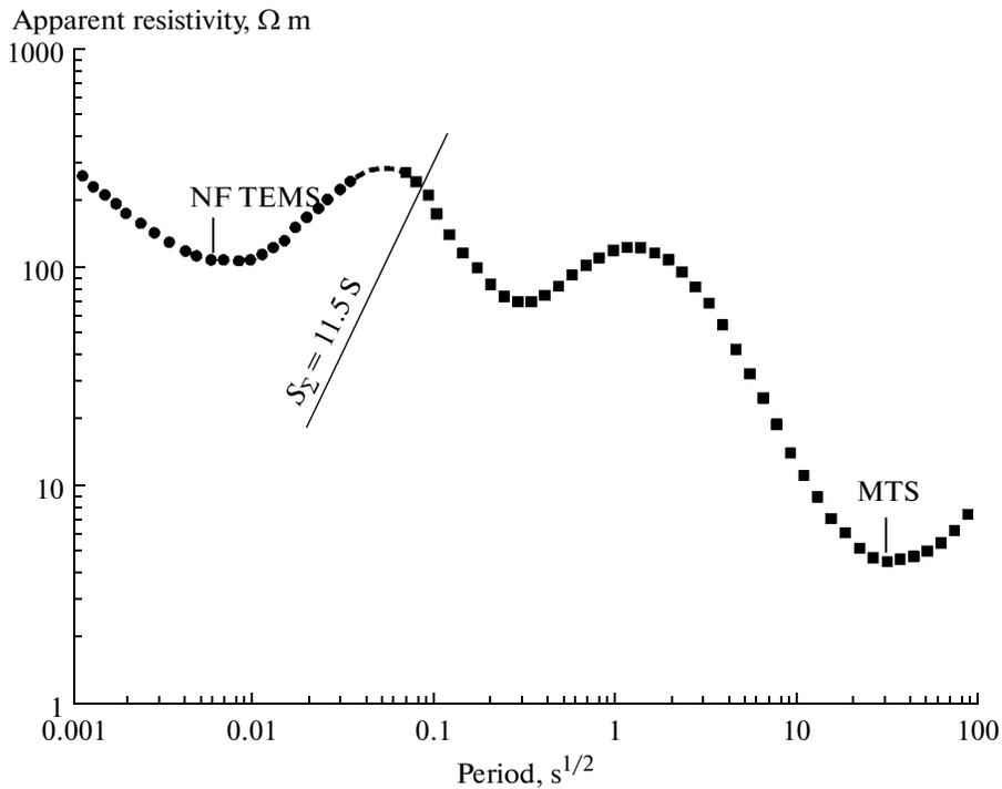
**Fig. 8.** Example of alignment of the NF TEMS and MTS curves at the single sounding site.
