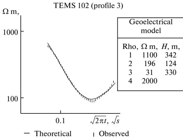
**Fig. 2.** Field data, synthetic curve, and geoelectrical model at NF TEMS 102 (profile 3).
