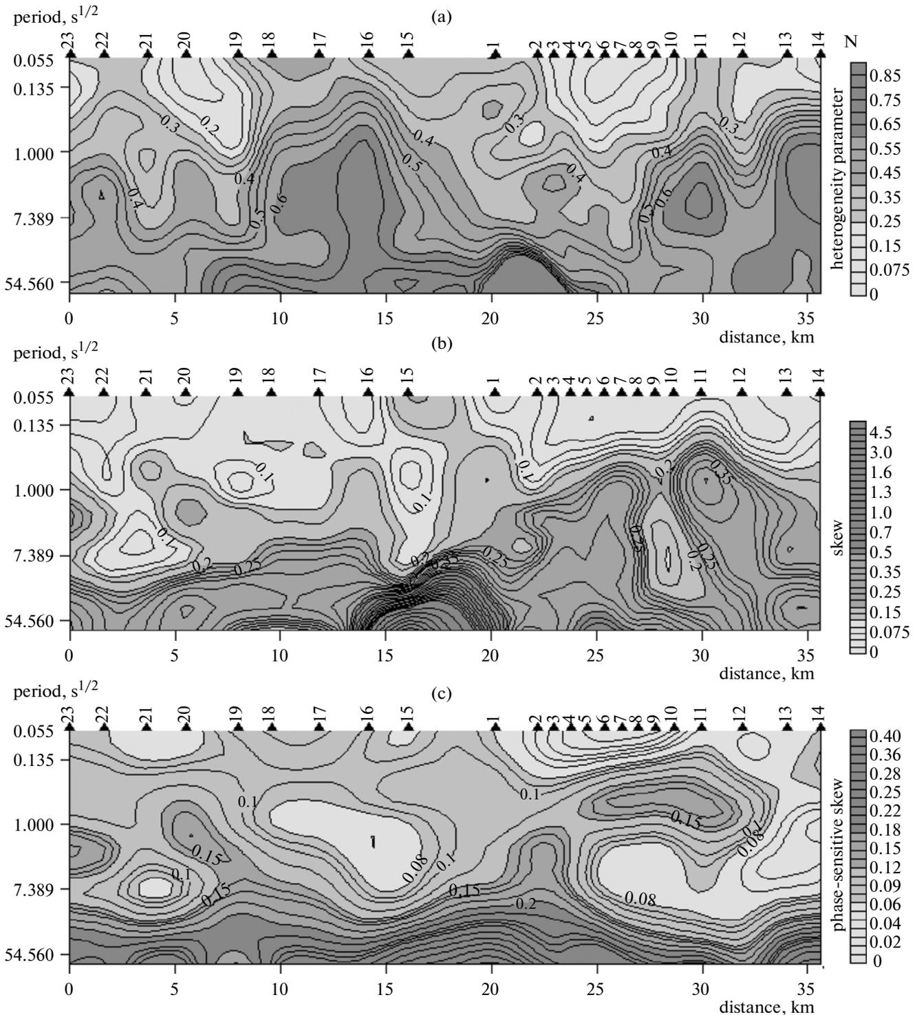
**Fig. 5.** Frequency sections of the magnetotelluric parameters: (a) heterogeneity parameter  $N$ ; (b) skew; (c) phase-sensitive skew  $\eta$ .
