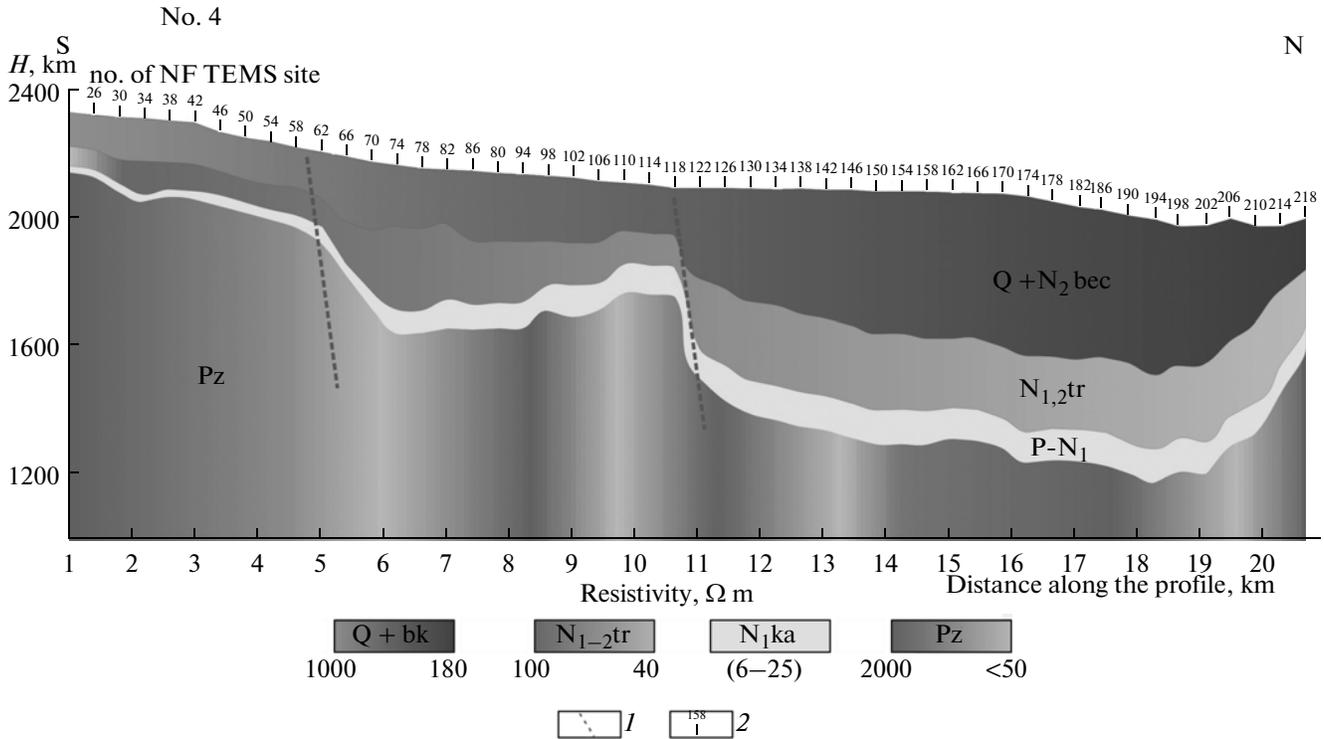
Fig. 11. Geoelectrical section along profile 4, according to the NF TEMS data: 1 supposed faults; 2 NF TEMS and MTS sites.
