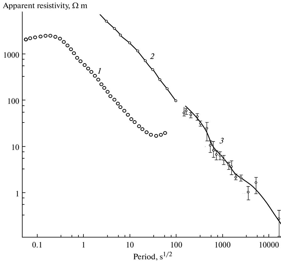
**Fig. 7.** Position of the observed MTS curve relative to the normal Vanyan's curve and the global magnetovariational sounding curve. (1) Vanyan's global curve; (2) MVS; (3) experimental data.
