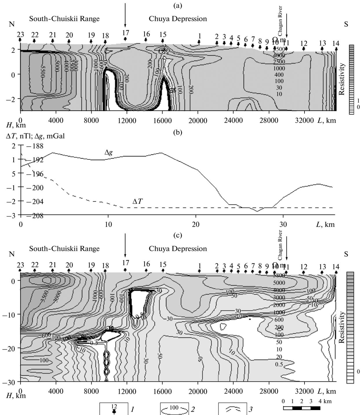
**Fig. 10.** (a) Geoelectrical section of the sedimentary cover along profile I-I; (a) upper part of the geoelectric section; (b) graphs of gravity and magnetic field; (c) deep geoelectrical section along profile I-I: 1 sites of magnetotelluric sounding; 2 equiresistivity contours in  $\Omega$  m; 3 graphs of gravity and magnetic fields.
