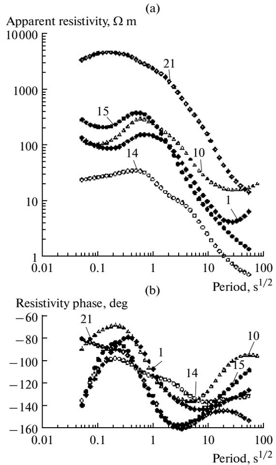
Fig. 6. Typical longitudinal MTS curves along the profile I-I: (a) amplitudinal; (b) phase.
