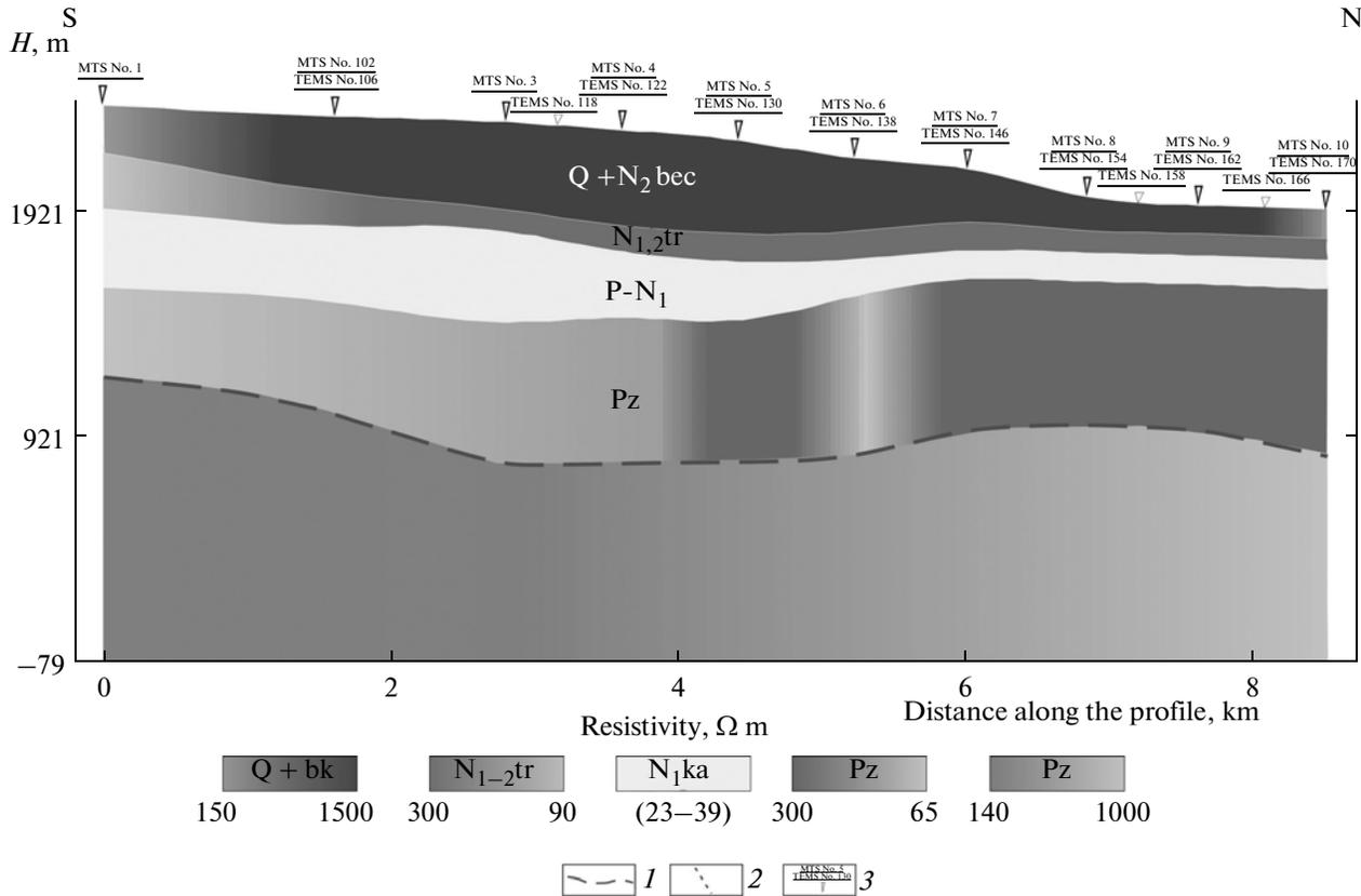
**Fig. 9.** Geoelectrical section along profile 3, according to the joint interpretation of NF TEMS and MTS data: 1 geoelectrical boundary in the basement; 2 supposed faults; 3 NF TEMS and MTS sites.
