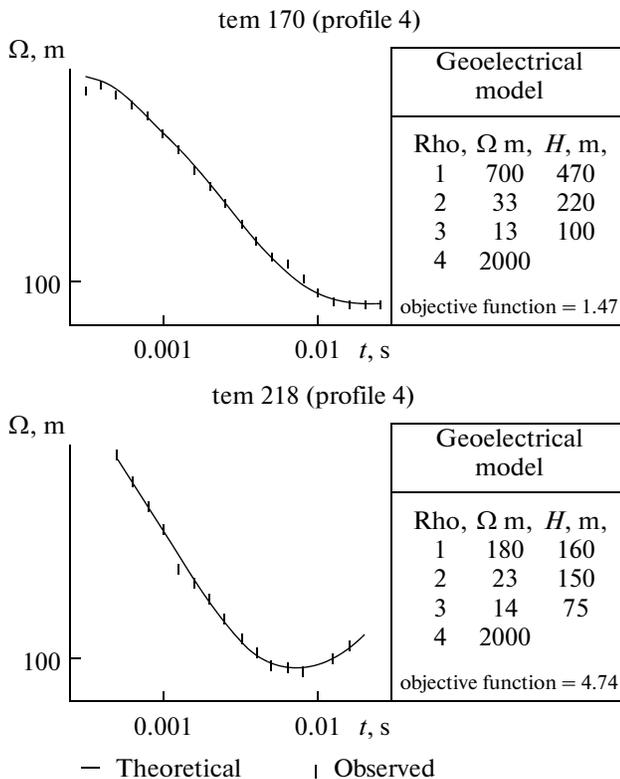
**Fig. 3.** Field data, synthetic curves, and geoelectrical models at NF TEMS 170 and 218 (profile 4).
