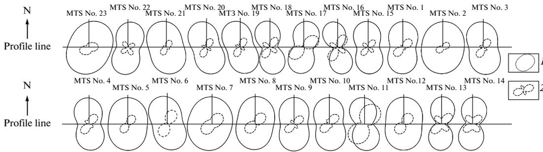
Fig. 4. Polar diagrams of the impedance tensor  $|\hat{Z}|$  for the period  $T = 1$  s: 1 polar diagram  $|Z_{xy}|$ ; 2 polar diagram  $|Z_{xx}|$ .
