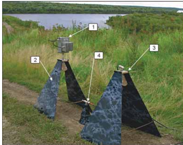
Fig. 3. General view of the receiving and transmitting equipment for UWB EMP sounding: 1, electromagnetic pulse generator based on DSRDs; 2, UWB bi-leaf microstrip transmitting antenna; 3, receiving antenna similar to 2; 4, UWB monopole receiving antenna.
