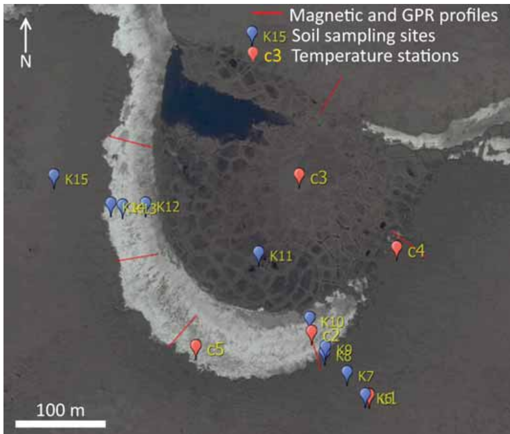
Figure 2.19-18: Ancient time drained alas: soil sampling sites, GPR and magnetic profiles, temperature stations
