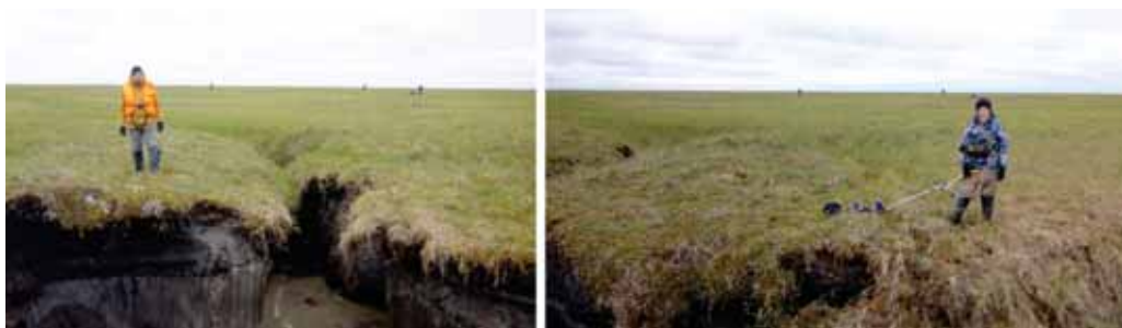
Figure 2.19-14: Erosional gully (left); GPR with 700 MHz antenna (right); studying area is on the background on both photos
