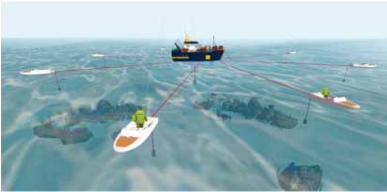
Figure 7 Deployment of a floating CED system.
